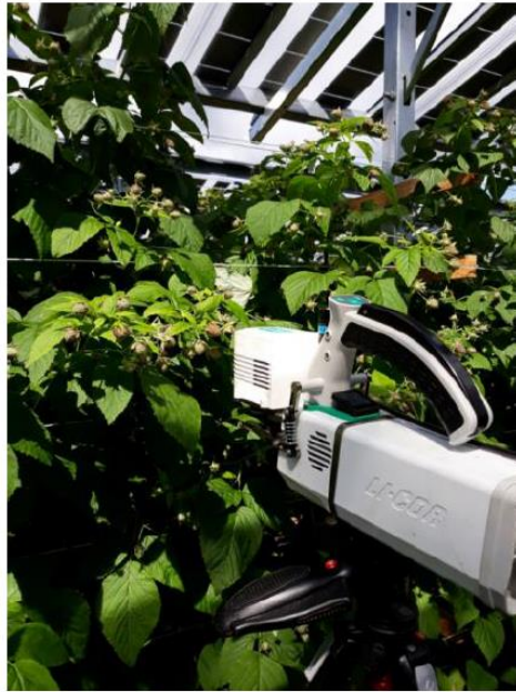
Figure 4. The measurement head of the LICOR LI6800 Photosynthesis measurement system, attached to a raspberry leaf.
